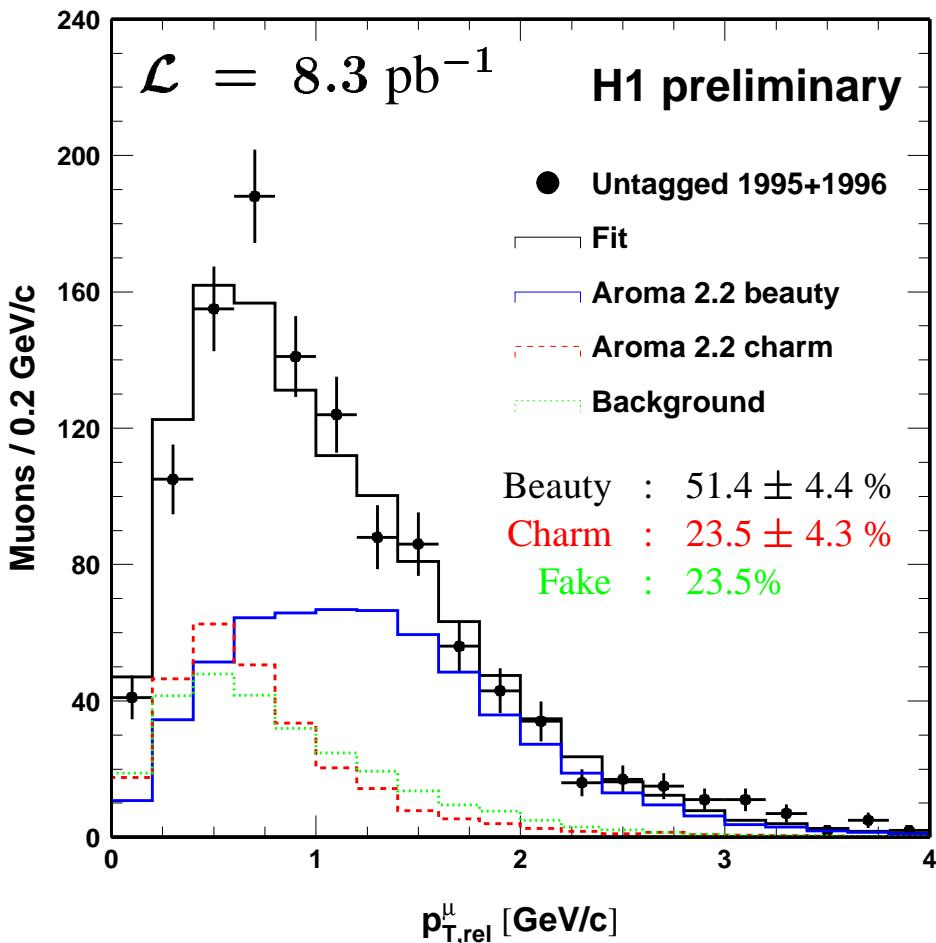
$$\sigma_{b\bar{b}}^{vis} = 0.93 \pm 0.08 {}^{+0.21}_{-0.12} \text{ nb (H1 prel.)}$$
