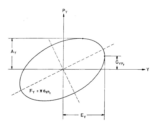
Figure 4: Projection on the  $y-p_y$  plane;  $(y\equiv x,z,\sigma)$
