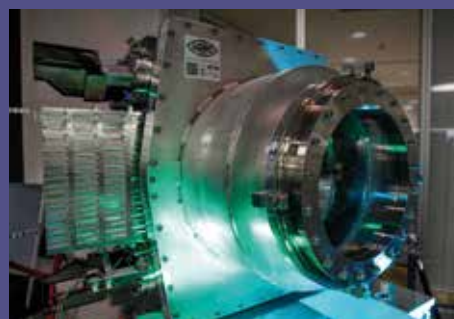
The Adaptive Gain Integrating Pixel Detector (AGIPD), tailor-made for the European XFEL, can record the world’s fastest X-ray serial images.
