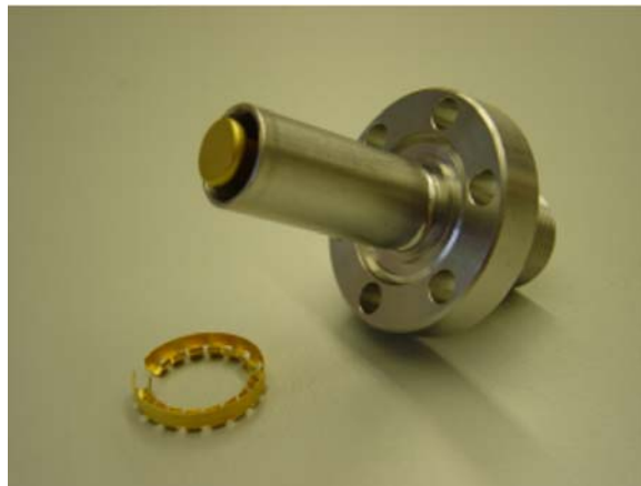
FIGURE 4. Pick-up electrode for the 34 mm FLASH button BPM
