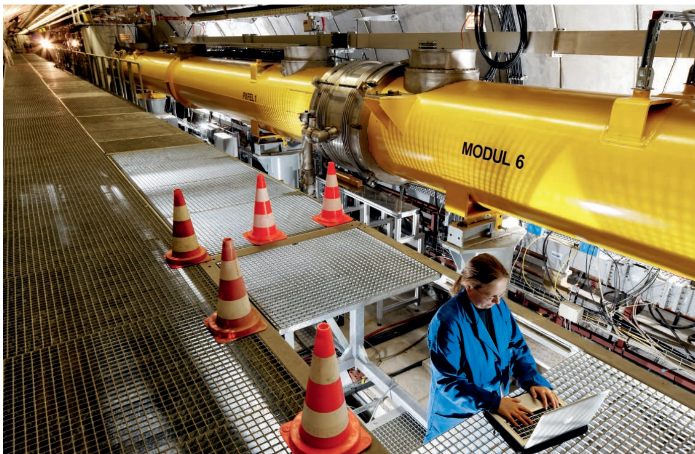
A real racer: The FLASH free-electron laser accelerates electrons to high speeds and uses them to generate ultrashort X-ray laser flashes. Picture: Heiner Müller-Elsner / DESY
