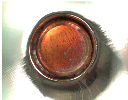
FIG. 6. Photograph of the inner surface of the back wall of a photoinjector cavity with inserted copper cathode plug.
