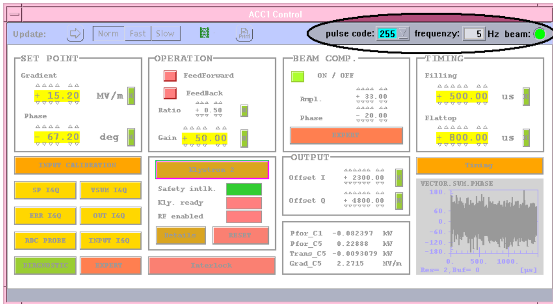
Figure 9: A panel for a component displays only data and settings for the pulse code specified in the upper right corner. Changes of parameters affect only the operation of the pulse code specified.
