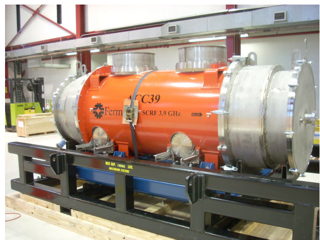
Figure 10: ACC39 on its shipping mount prior to shipment. The base frame is black and the isolation frame upon which the module is directly placed is blue.
