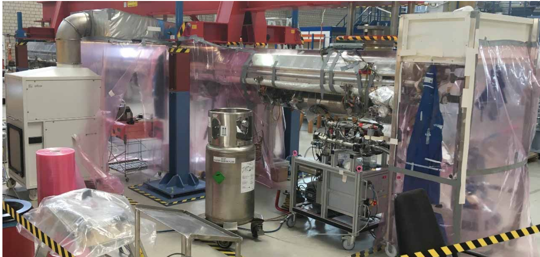
Figure 2: Module PXM3.1 C6 FPC cold part exchange in a local clean room (center left) in AMTF (June 2022).
