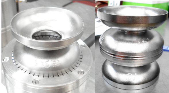
Figure 3: Equatorial weld lip preparation of the dumbbells (left) and samples (right) for equatorial EBW parameters.
