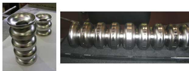
Figure 1: Components of the Nb mockup during intermediate fabrication steps.
