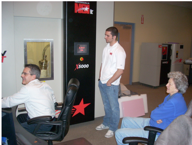
Figure 4: 3.9 GHz cavity undergoing X-ray scanning at NorthStar Imaging, Inc.
