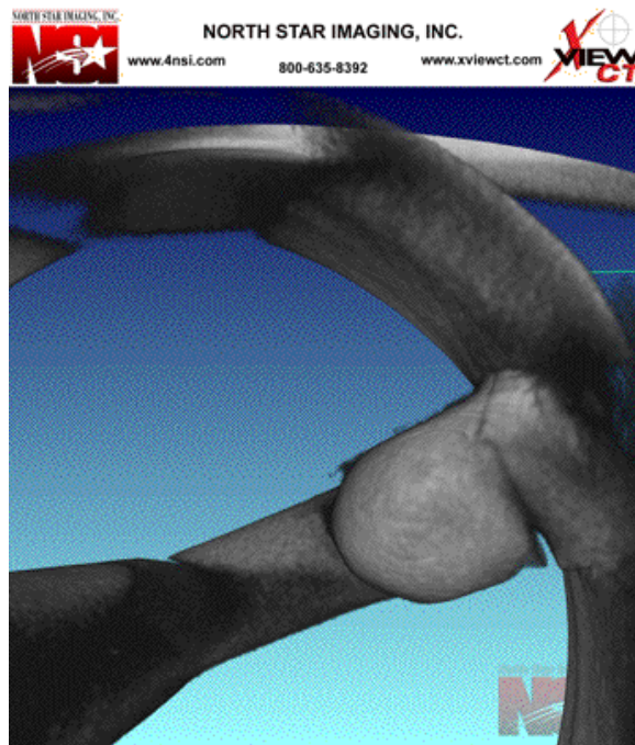
Figure 3: Fractured Formteil on Cavity F3A6 as determined using 3-D, X-ray computed tomography.
