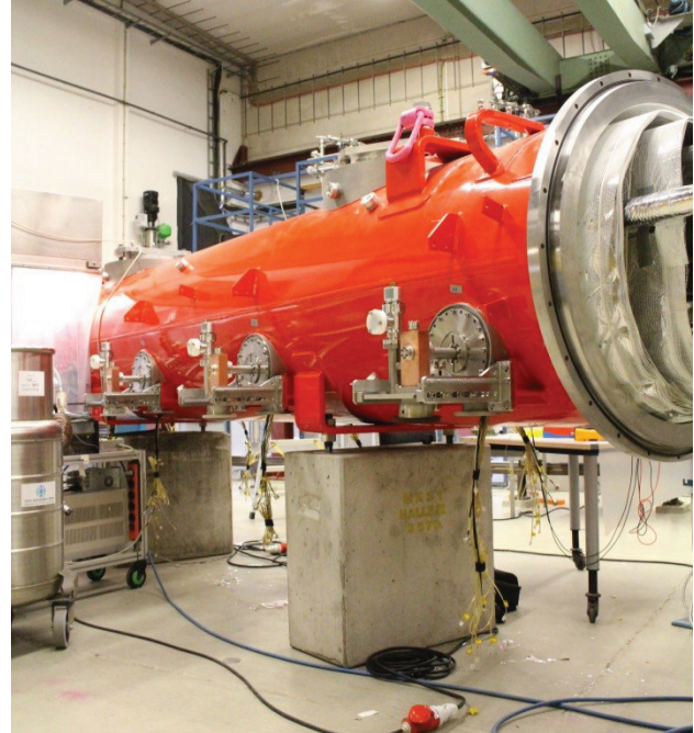
Figure 6: The X3M1 during Warm Coupler parts installation.
