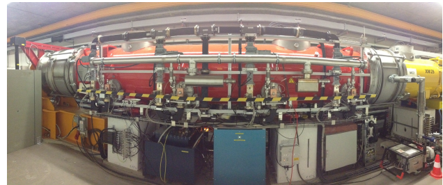
Figure 1: The third harmonic module with eight cavities inside at the injector of the E-XFEL.
