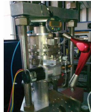
Figure 9: Setup for testing 3.9 GHz coaxial tuner units.
