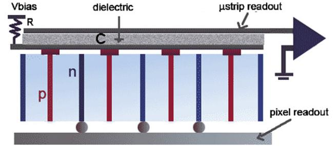
Fig. 3. Sketch of one of the possible dual electrode readout configurations showing a pixel bump-bonded readout at the bottom and bias electrode microstrip readout on top. The resistor,  $R$ , keeps the low-impedance bias supply from shorting out the signal, allowing it to be coupled through the capacitance,  $C$ , of the dielectric to the readout line. The electrodes extend to the field oxide layers (not shown).
