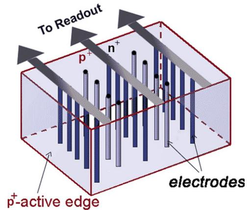
Fig. 4. Three-dimensional schematic view of a same-side strip and pixel readout. The bumps to the pixel readout chip (not shown) are represented by the black dots on the  $n^+$  electrodes. The  $R$  and  $C$  of Fig. 3 are also needed but, for simplicity, are not shown here.
