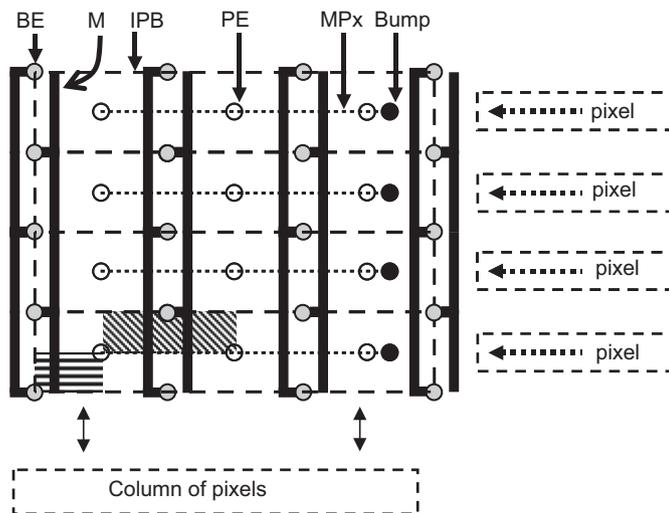
**Fig. 6.** Schematic diagram of a strip readout on the opposite side of a pixel readout to subdivide each pixel into 6 sub-parts (2 are shaded). (BE) bias electrodes, (M) strip readout, (IPB) dashed lines—inter-pixel boundaries, and, on the other side, (PE) open circles—pixel signal electrodes, (MPx) dotted lines—connecting metal, (Bump) bump bonds. The  $p^+$  implants, shown in Fig. 5 are also used here on both sides, but not explicitly shown to keep the diagram uncluttered.
