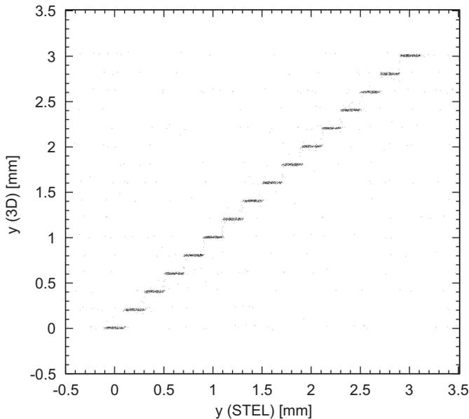
**Fig. 1.** Correlation between the hit positions  $y(3D)$  measured by the 3D detector and the predicted track position  $y(STEL)$  showing the spatial resolution comparison between the telescope and 3D detecting elements.
