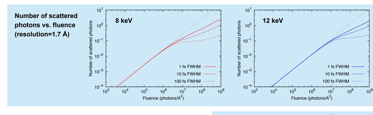
To describe the strength of the x-ray scattering signals, the number of scattered photons limited to the desired spatial resolution length *d* is given by
