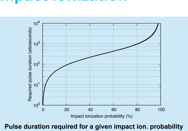
Another important damage mechanism characteristic of extended molecular systems is impact ionization by (quasi-)free electrons. For an x-ray pulse much shorter than inner-shell decay lifetimes, impact ionization by Auger electrons is irrelevant, but impact ionization by photoelectrons is not negligible. By using short pulses, one can suppress photoelectron impact ionization.
