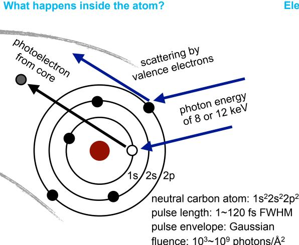
Since the electronic damage processes are mainly atom-specific in the x-ray regime, one may concentrate on the interaction of the x rays with individual atoms. Even if the atomic motion during an x-ray pulse is negligible, electronic damage (photoionization and
