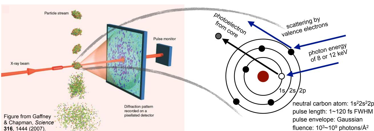
Single-shot imaging employs coherent x-ray scattering to determine the atomically resolved structure of non-crystallized biomolecules or other nanoparticles, with the high fluence of a tightly focused x-ray FEL pulse that could produce a significant amount of scattered
