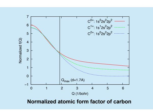
To examine variations of x-ray scattering patterns for different electronic configurations, especially for core-hole configurations created via photoabsorption, we calculate atomic form factors for the filled core (neutral: 1s<sup>2</sup>2s<sup>2</sup>2p<sup>2</sup>), the single-core-hole (1s<sup>1</sup>2s<sup>2</sup>2p<sup>2</sup>), and the double-core-hole (1s<sup>0</sup>2s<sup>2</sup>2p<sup>2</sup>) configurations.
