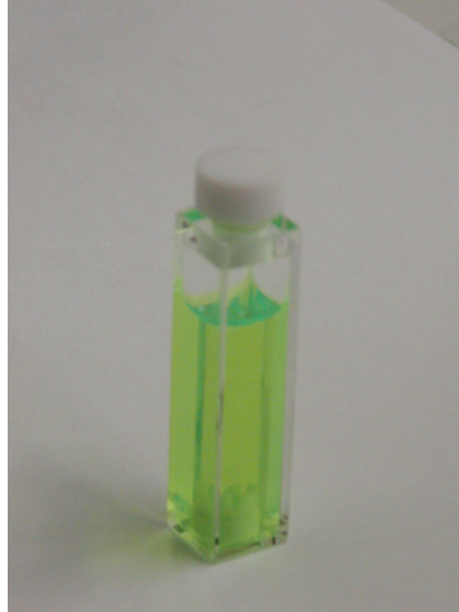
Figure 4.6: The dye is stored in this cuvette on the dye module inside the Laser box. The cuvette volume is 1.2\text{cm} \times 1.2\text{cm} \times 5\text{cm}
