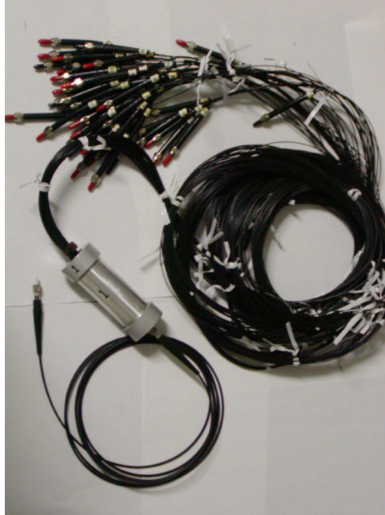
Figure 4.11: The sub-splitter. It is used in the detector area to split the light for each detector (directly PMT in some cases). This is 1 \times 49 splitter, the same type as is installed for the calorimeter.
