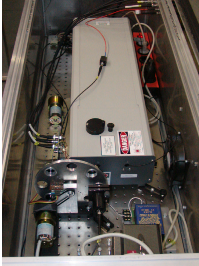
Figure 4.4: The layout inside of Laser "coffin". The white box in the center of this picture is the Laser module (Laser box). The motorized filter wheel is placed in the lower left with the DC-motor.
