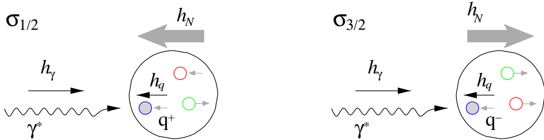
Figure 2.8: Schematic of polarized DIS. The virtual photon helicity h_\gamma , quark helicity h_q and nucleon helicity h_N are indicated in the figure.
