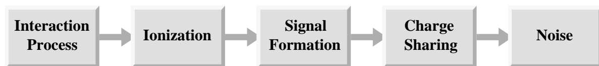
Figure 3.11: Different steps that transform an energy deposition straggling function into an observed ionization straggling function.
