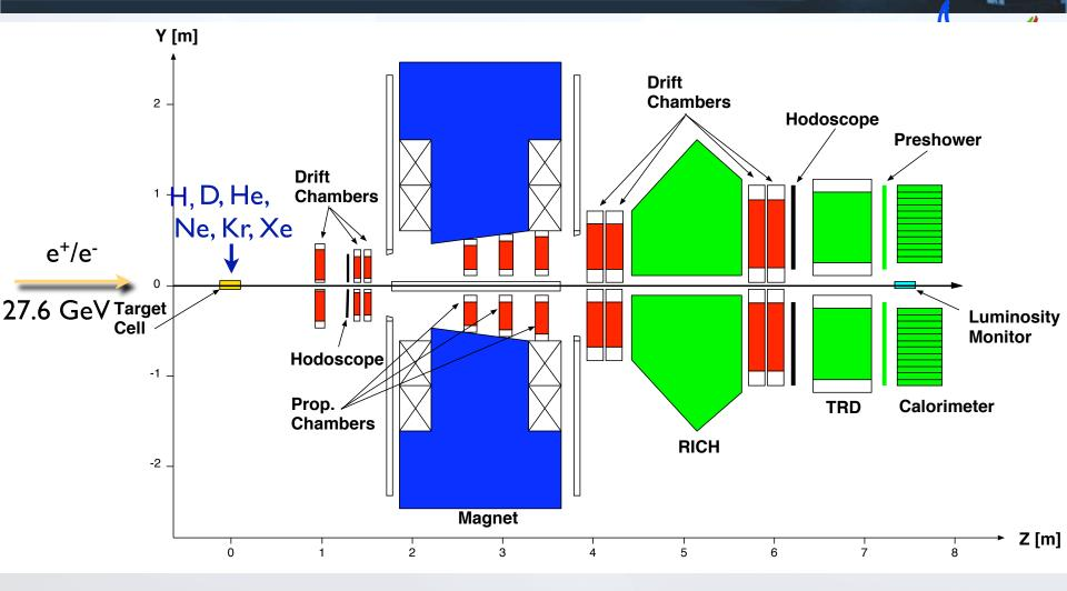
Magnetic spectrometer with transv. and long. polarized targets
