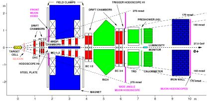
BeamLong. pol.  $e^{\pm}$  at 27.6 GeVLep.-Had. Sep.High efficiency  $\approx 98\%$ TargetTrans. pol. H ( $\approx 75\%$ )Low contamination (<2%)</th>Log. pol. H ( $\approx 85\%$ )Hadron PIDSeparates  $\pi^{\pm}, K^{\pm}, p, \bar{p}$ Unpol. H,D,Ne,Kr,...with momenta in 2-15 GeV
